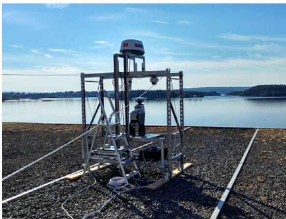
Figure 13: DNV GL test rig for testing the performance of sensors for condition detection
